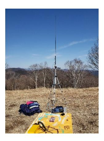
The appeal of CW is that it allows long distance communication with simple equipment. Recently, I've also become interested in QRP operation, and I've realized that it works surprisingly well even with an output of less than 5W. My favorite rigs are IC-705 and KIT QRP machines, and I mainly operate on the 10 MHz band.
