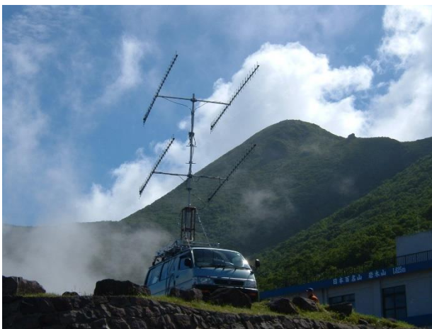
Mobile operation in Mt. Iwaki, using stack antennas of 430MHz
