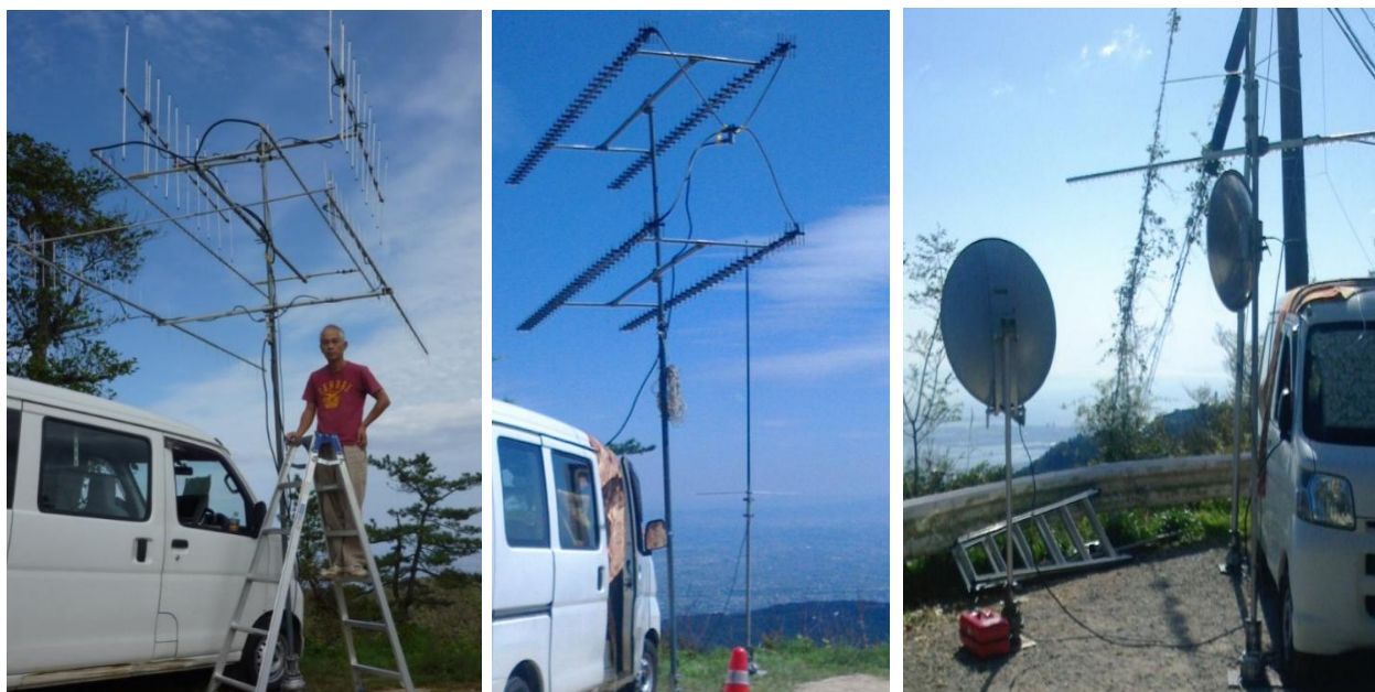
Right: Antennas for 144, 430 and 1200MHz. Middle: Only for 1200 MHz Left: Parabolic antennas for 2400 and 5600 MHz bands.
