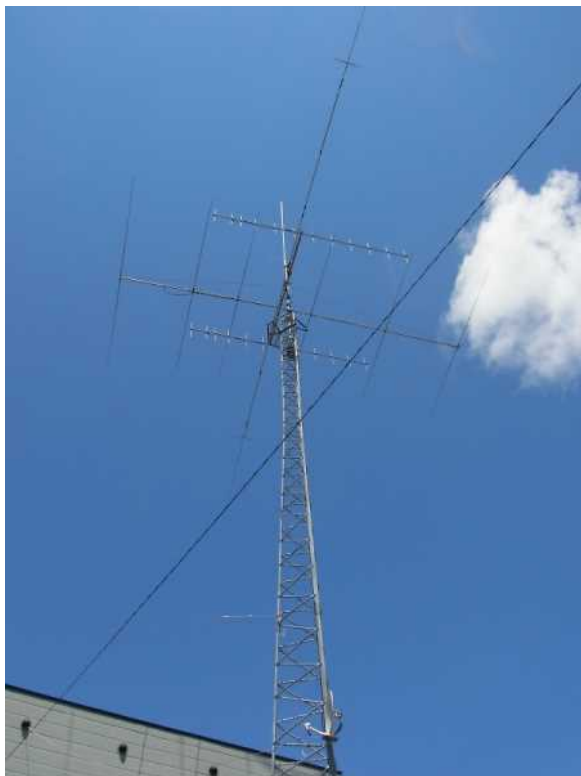
Top to bottom: 144MHz GP, 3.5 MHz CD-78, 144MHz Yagi stack, 28MHz 6ele Yagi
